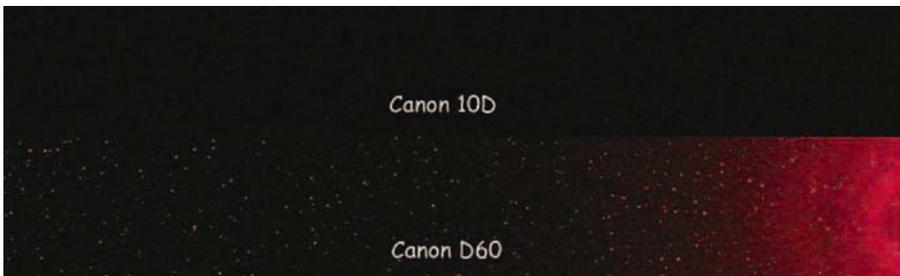
**Figure 5.3.** Comparison image of the noise performance – Canon 10D vs. D60.
